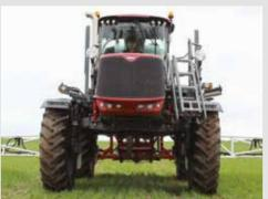
62001 Engine: Cummins 300 hp Transmission: 4WD hydrostatic transmission Topcon X35 Controller: Chem transfer: 35L TurboFiller 1.45 metre Clearance: Track width: 3 - 3.5 metre TR5 36.5-42.5m, Boom: B3 Mega 48.5m TERRA FORCE 36.5-42.5m Pump: 650 l/m Run Dry centrifugal pump
